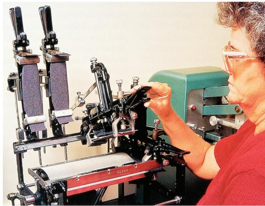
On the Wyzenbeek machine the blue-gray strips of fabric are the test specimens held in place by the arms that will be lowered to oscillate over the cotton duck-covered cylinder below.
